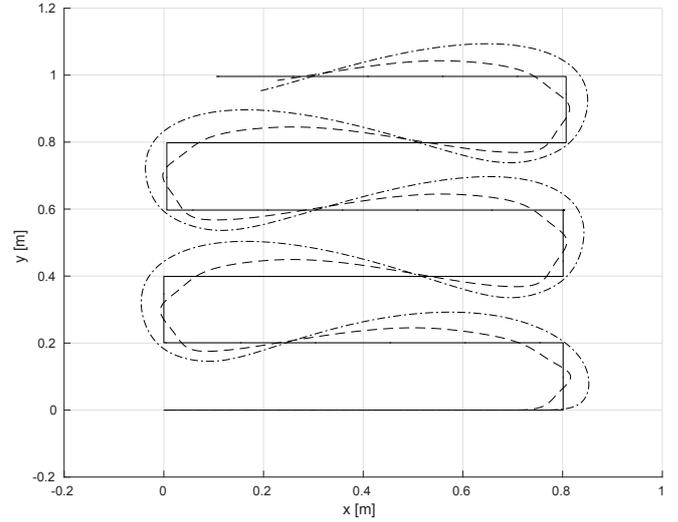
Figure 3. Trajectory of quadrotors motion (dashed), load (dotted) and referenced trajectory (solid) with full controller
