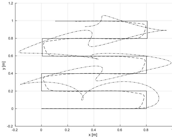
Figure 2. Trajectory of quadrotors motion (dashed), load (dotted) and referenced trajectory (solid) with partial controller
