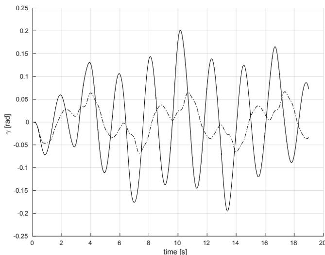
Figure 6. Angle  $\gamma$  oscillations with full controller (dotted) and with partial controller (solid)
