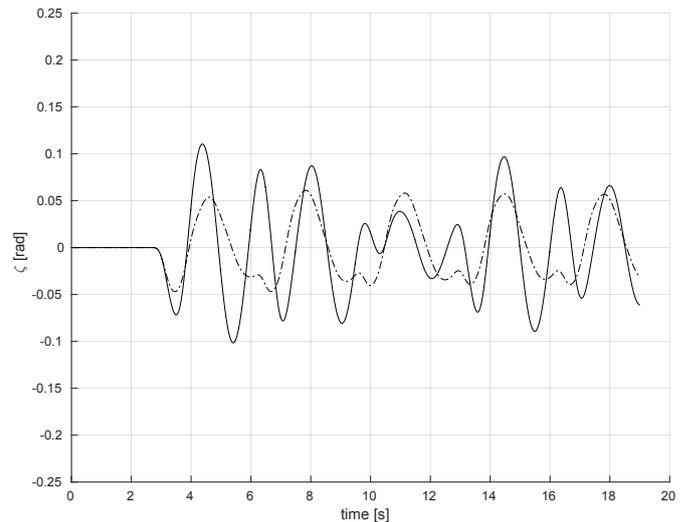
Figure 7. Angle  $\zeta$  oscillations with full controller (dotted) and with partial controller (solid)
