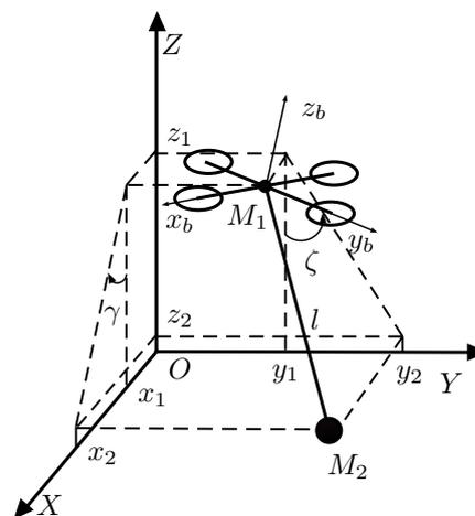
Figure 1. Quadrotor with a payload on suspension.
