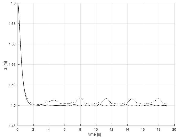
Figure 4. Quadrotor altitude change with full controller (dotted) and with partial controller (solid)
