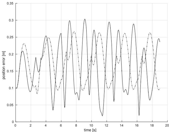
Figure 5. Path control error change with full controller (dotted) and with partial controller (solid)
